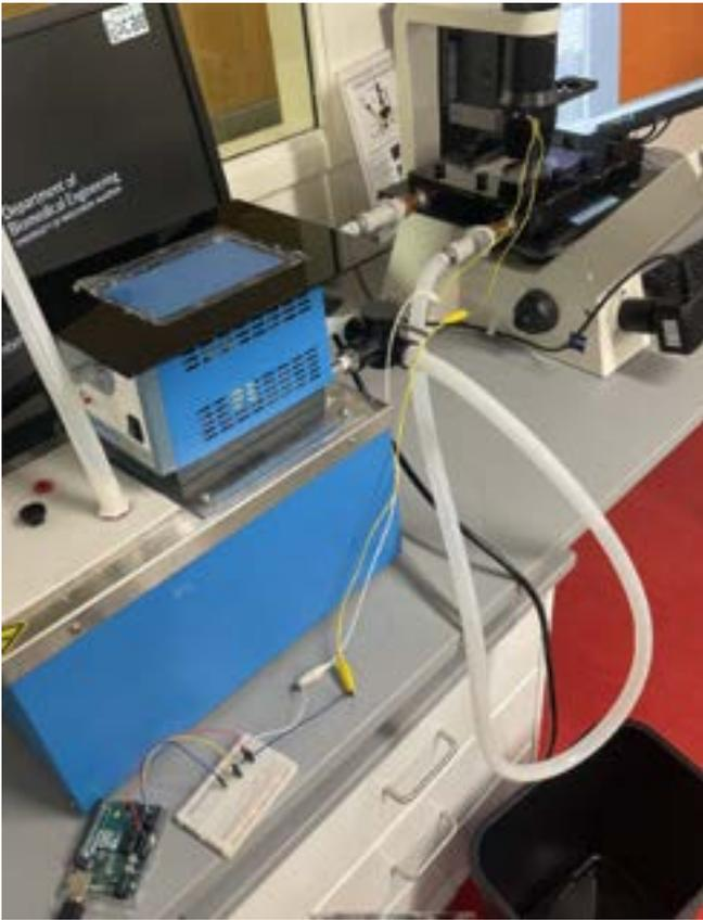
*Figure 2: Homogeneity testing for temperature whole set up.*
