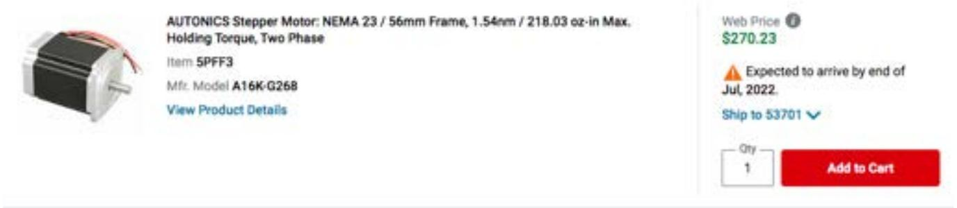
**AUTONICS Stepper Motor: NEMA 23 / 56mm Frame, 1.54nm / 218.03 oz-in Max. Holding Torque, Two Phase**
