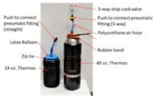
Fig 2. Dry ice storage containers for providing CO<sub>2</sub> to the incubator. The thermos that can store dry ice while providing CO<sub>2</sub> to the incubator. The capacity to store more dry ice in a larger thermos allows uninterrupted use for over four days.
