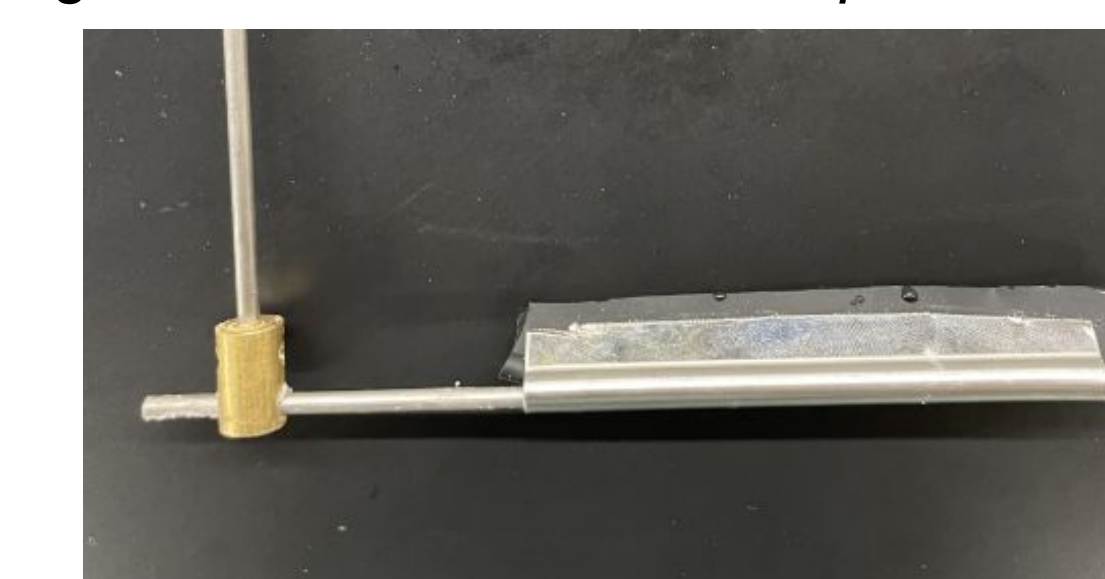
Figure 7: Fabricated preliminary wiper blade
