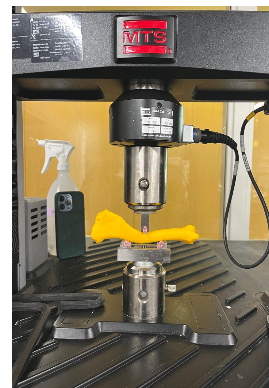
Figure 7. Image depicting the MTS performing a 3-point bend test on the 3D printed canine femur.
