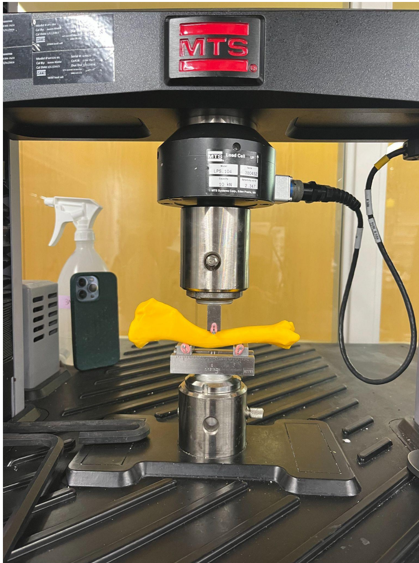
Figure 16. MTS machine with the 3 point bend fixture testing the final femur in compression
