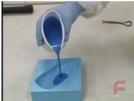
Figure [1] Pouring of silicone rubber into a mold
