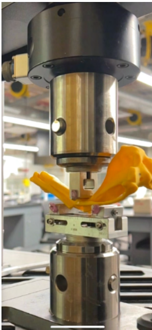
Figure 5: Model right after failure. The model underwent very little plastic deformation prior to fracture.
