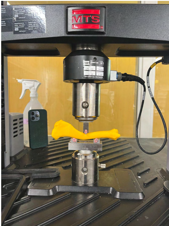
Figure 1: MTS Testing to determine peak load using a 3-point bend test.
