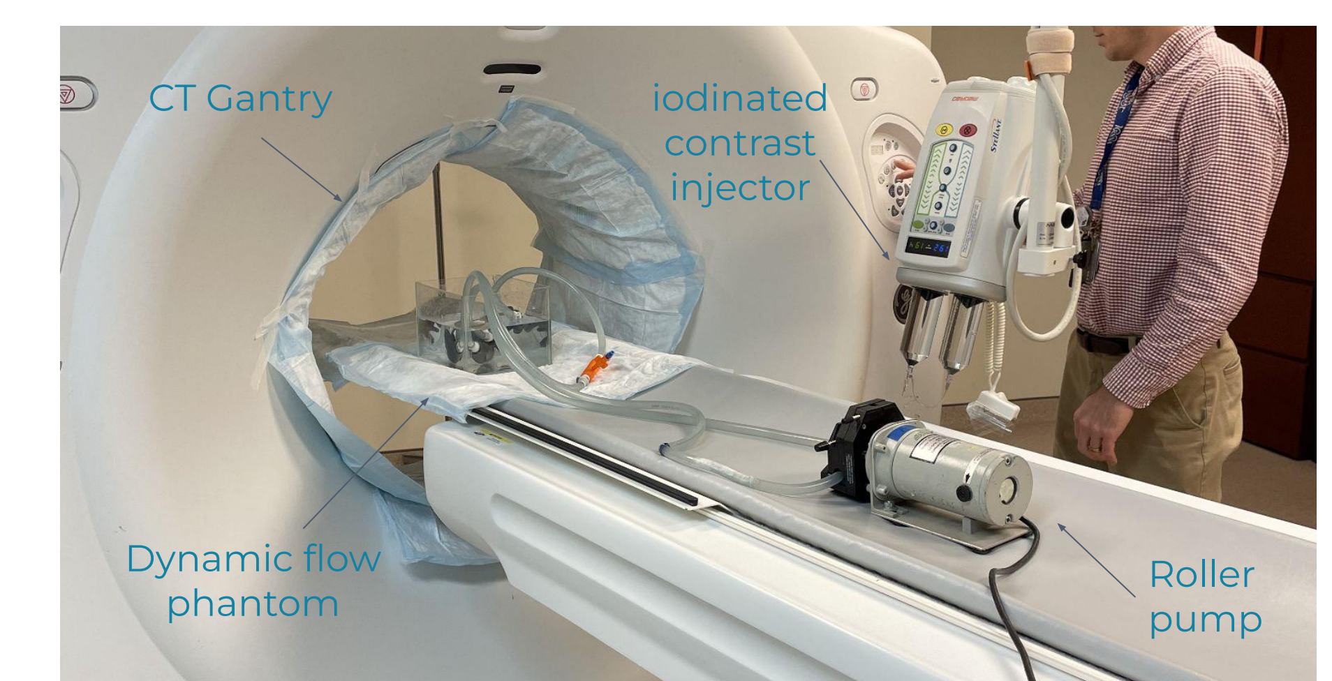
Figure 8: This image shows the phantom loading into the CT Machine
