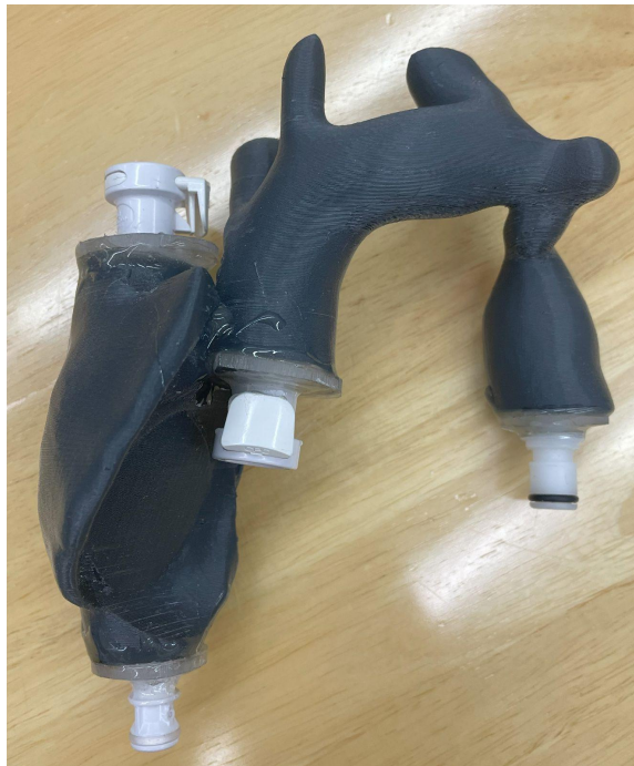
Figure 13: Printed heart phantom with connectors secured with Epoxy and clear acrylic to fill any gaps. The right atrium is on the left in the above image, and the ascending aorta is on the right.
