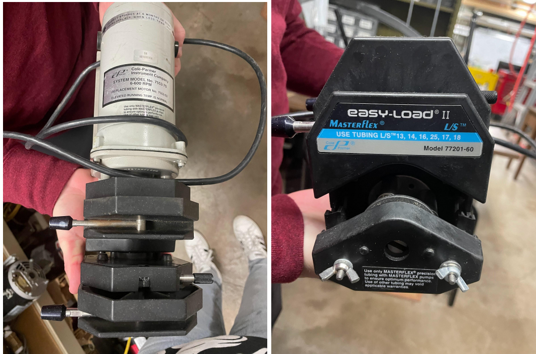
Figure 10: Roller pump borrowed from the UW Cardiovascular Fluid Dynamics Laboratory. The left image shows a top-down view with the motor information, and the right shows the roller pump information.
