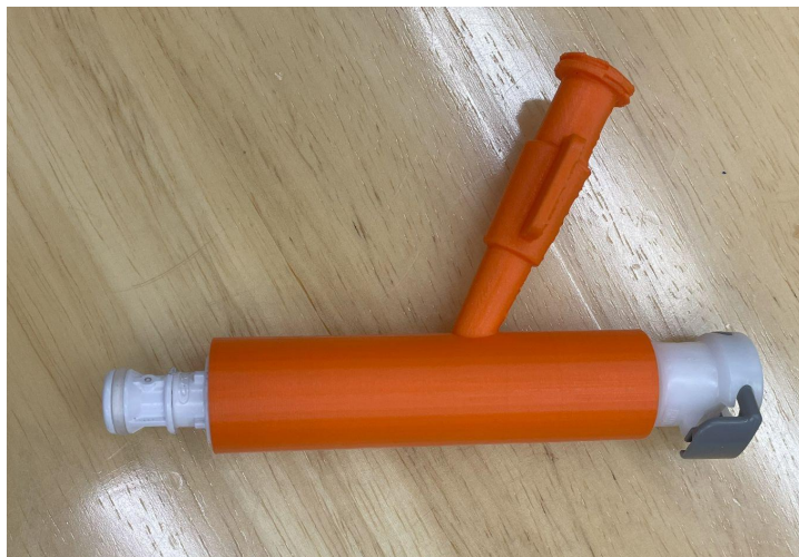
Figure 14: Printed injection site with connectors on both ends and the luer-lock extruding from the top.
