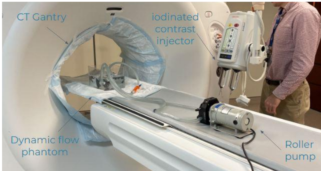
Figure 16: Complete flow phantom set up on the CT machine in the Wisconsin Institute for Medical Research Building for testing
