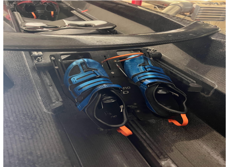
Figure 16: Picture of rowing shoes mounted onto footplate of boat
