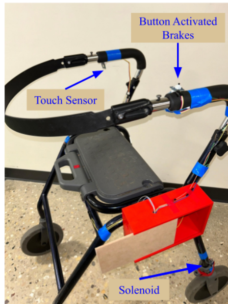
Figure 6: Isometric view of the final prototype, with button braking system on the near handle, touch sensor on the opposing handle, and solenoid in bottom right
