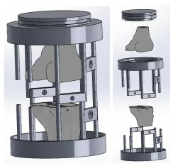
Figure 7. Completed assembly of prototype and exploded view
