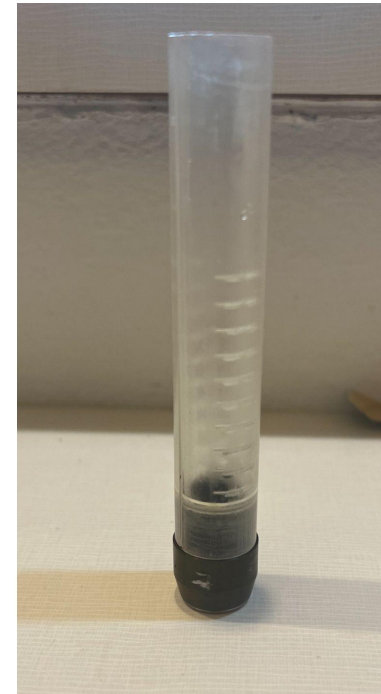
Figure 3: Current coring device prototype with a delrin plastic tube and 304 stainless steel blade.
