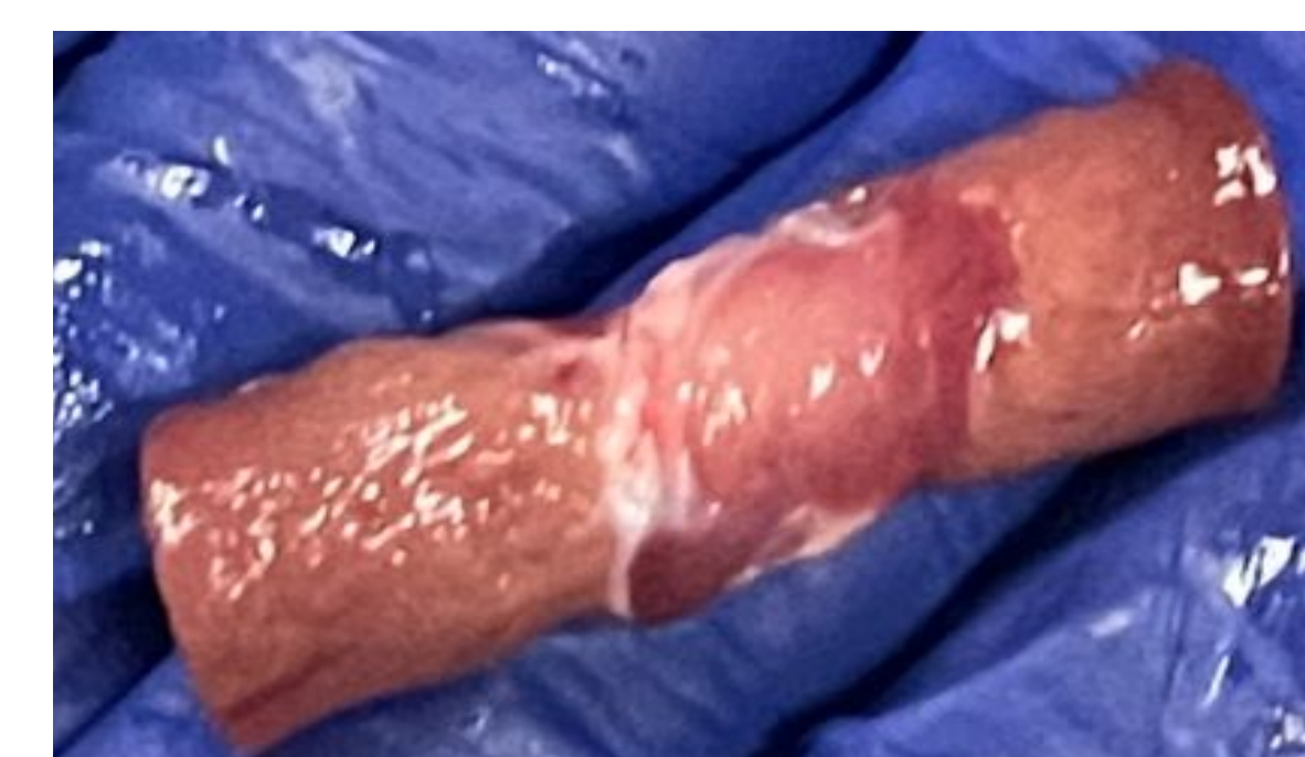
Figure 10: Image of staircase damage within internal tissue caused by Blade #3.
