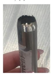
**Conclusions:** You will need more than just a belt sander to make the blade sharp enough. It is only feasible to make the blade thin enough without it flaking from overheating. We must look into alternate methods to sharpen the blade to ideal sharpness.
