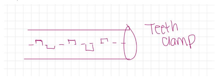
Figure 1: Teeth clamp design for coring tube
