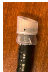
Figure 5: 3D printed endoscopic cap prototype on endoscope
