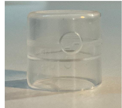
Figure 6 shown at top right favored cap design, less flexible material, longer viewing field and beveled end.
