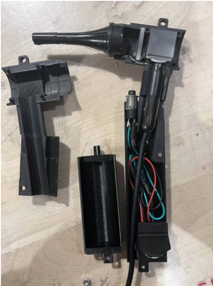
Internal of otoscope. Components: Magnifying lens, beam splitter, endoscope camera, button switch, microLED, CR2032 battery and holder, and additional wiring.
