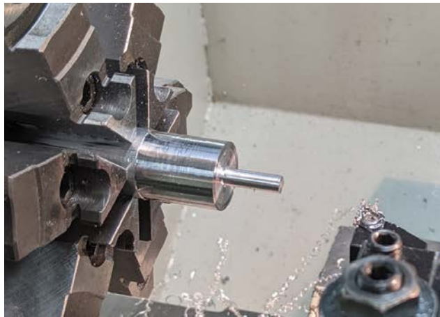
Figure 11: Turning the minor diameter (smaller end) of the device on the lathe.
