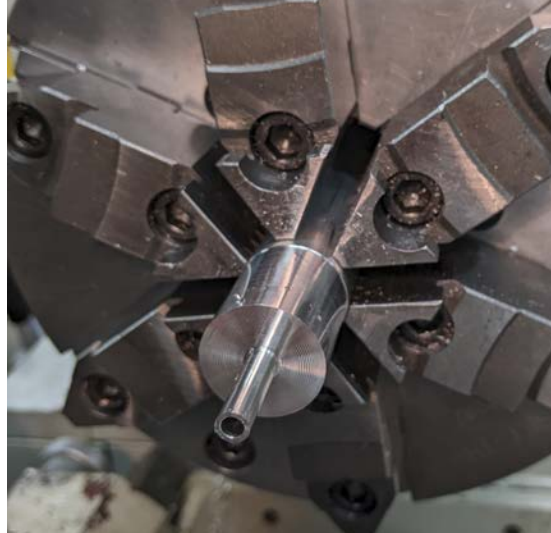
Figure 12: Drilling out the channel in the minor diameter of the device.
