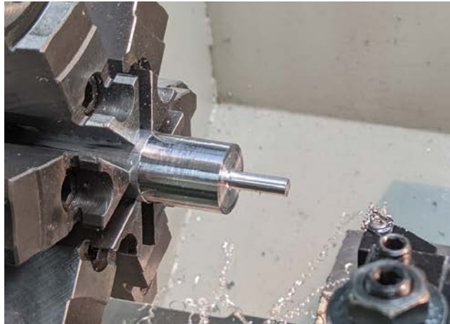
Figure B1: Turning the minor diameter (smaller end) of the device on the lathe.
