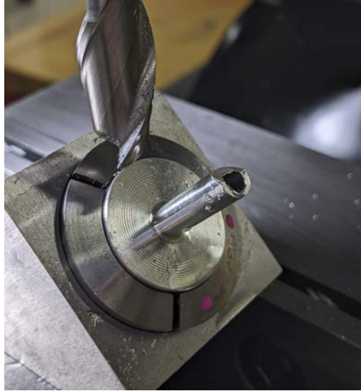
Figure 14: Using the mill to create the sharp angled edge of the device.
