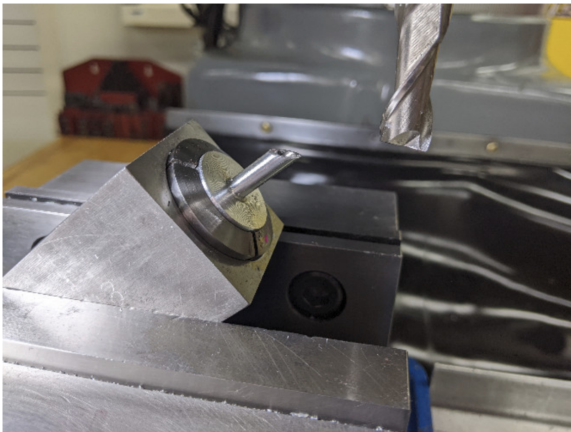
Finally, the piece was turned upside down and the small hole was drilled on the mill.
