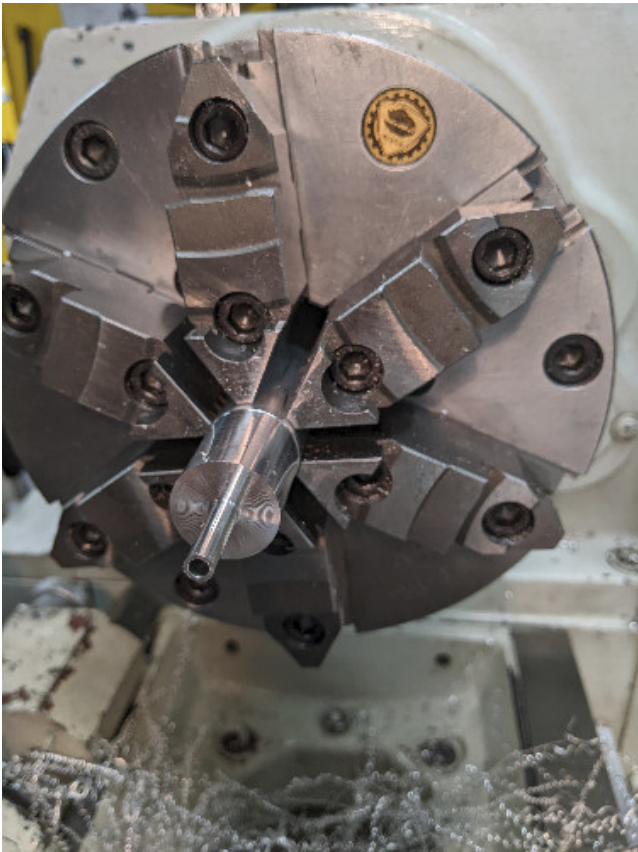
After that, the part was cut-off using the drop saw. The piece was then placed back into the lathe and the other end was drilled out. First with a normal bit, then a flat end mill.
