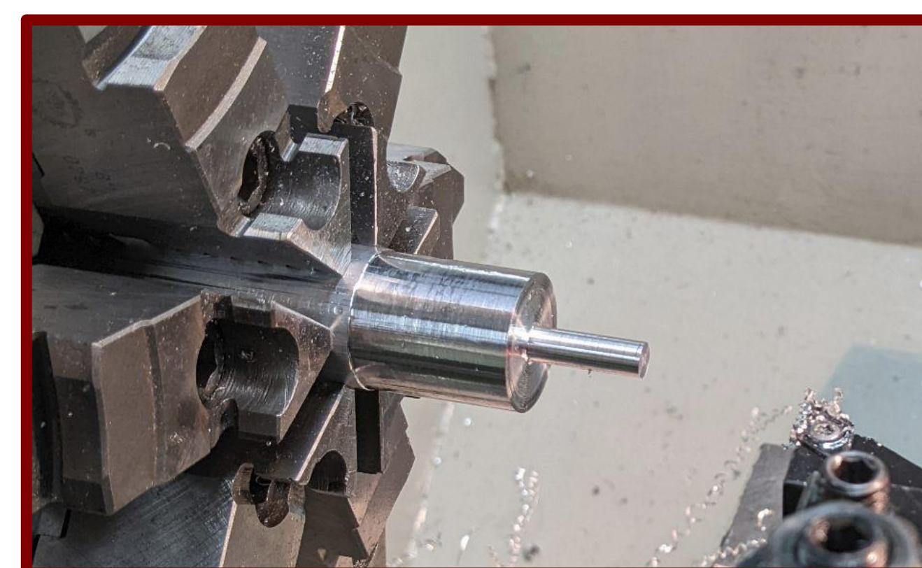
Figure 4: Turning on lathe to form overall shape and inner channel
