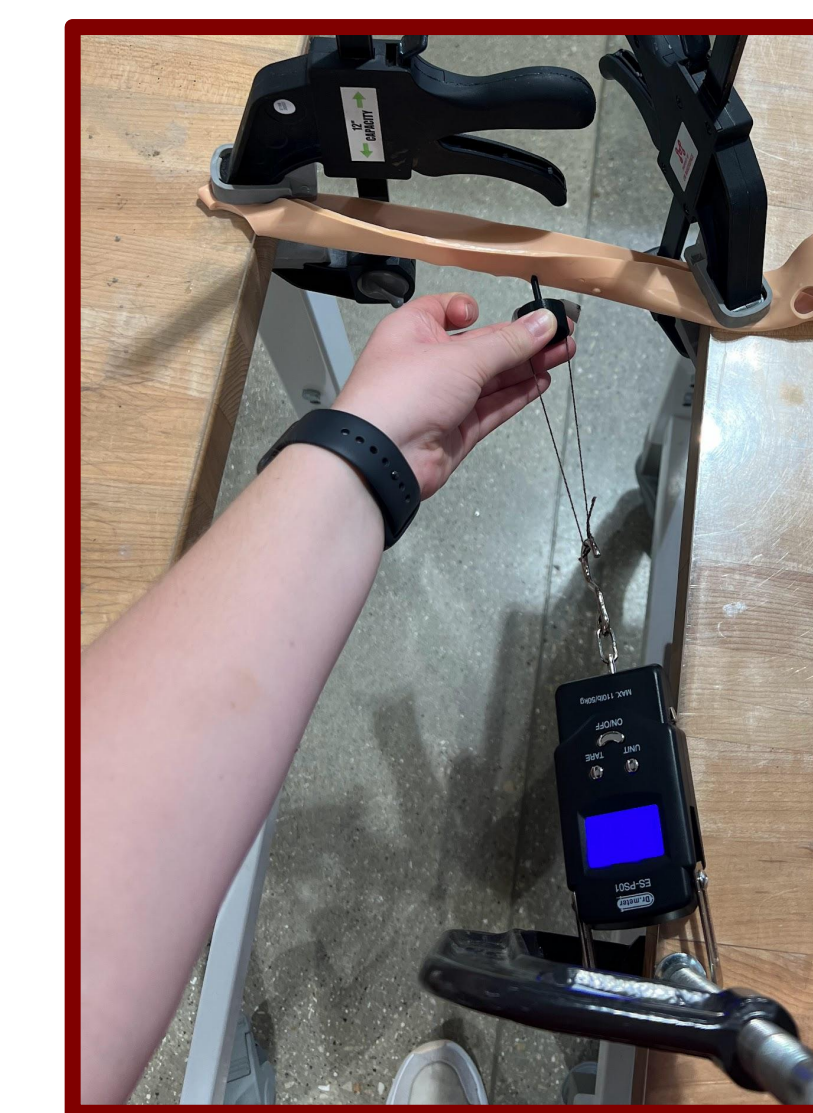
Figure 7: Skin puncture testing using force gauge
