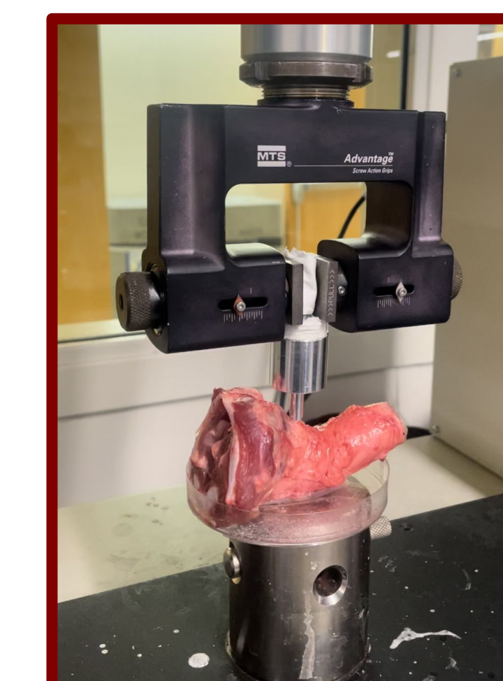
Figure 9: MTS testing of prototype with porcine larynx
