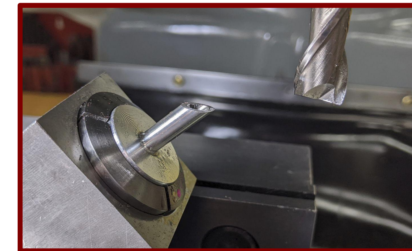
Figure 5: Using mill to create sharp cutting tip and additional hole
