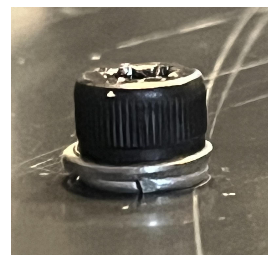
Figure 6: Testing with a standard washer above the split lock washer
