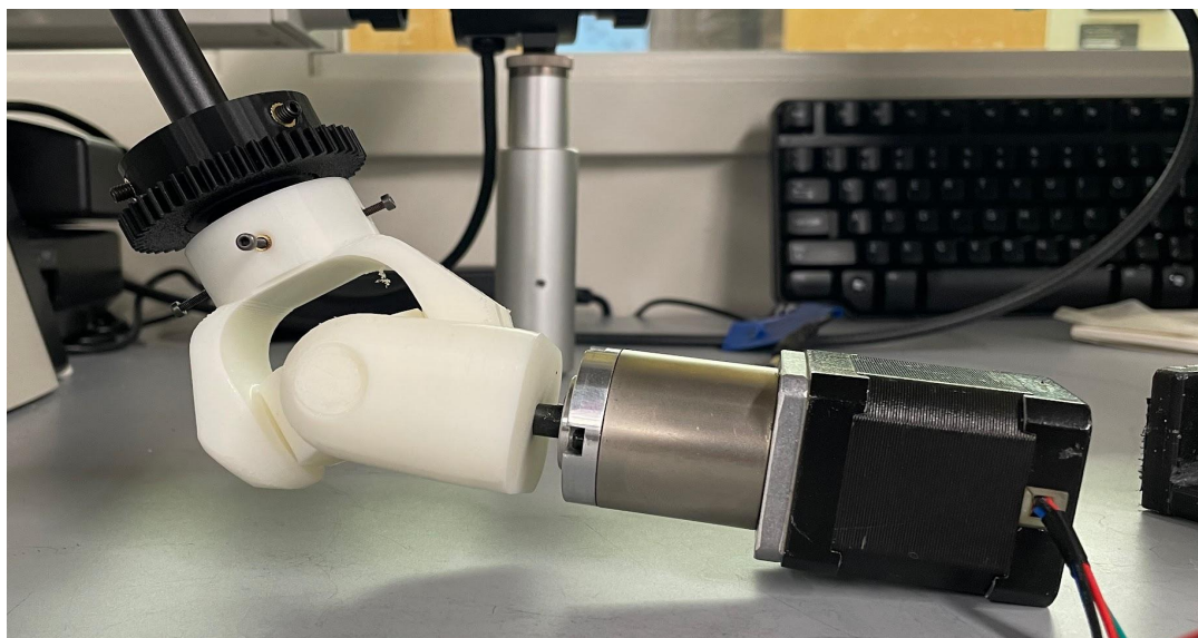
Figure 17: Direct connection testing set up. The universal joint connector is securely fastened to the x-axis manual control knob and the selected stepper motor.
