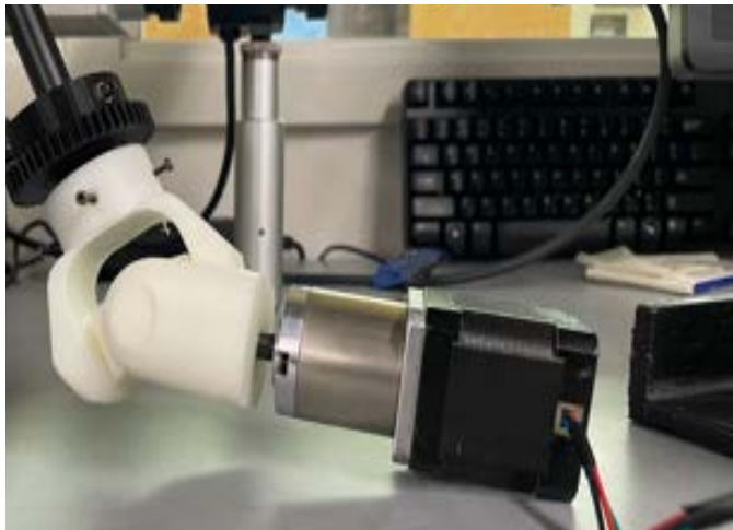
Figure 17: Direct connection testing set up. The universal joint connector is securely fastened to the x-axis manual control knob and the selected stepper motor.
