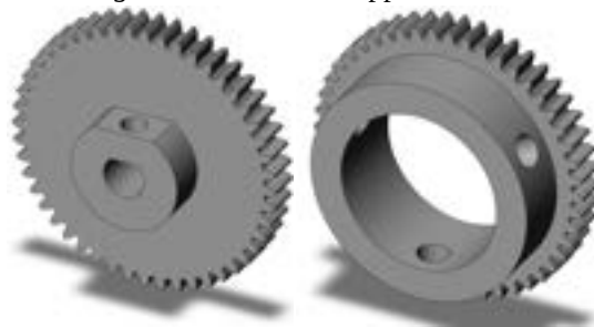
Figure 12: One of the knob gears (left) and one of the stepper gears (right).
