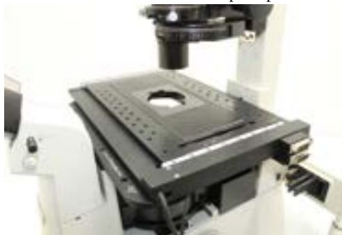
Figure 1: Nikon Ti-U Inverted Fluorescence Motorized Microscope [1].
