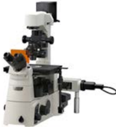
Figure 3: Nikon TI-U inverted fluorescence microscope used in the BME Teaching Lab [6]
