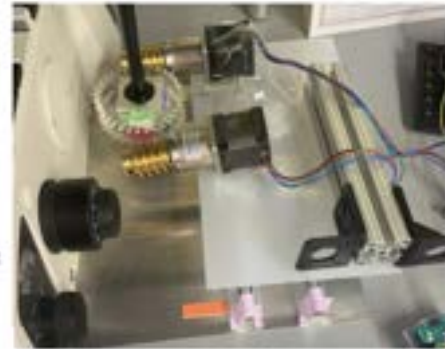
Figure 7. The mechanical part of the design. The stage knob with the gear attachment is shown on the left, with the stepper motors and worm drive gears.
