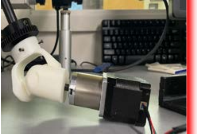
Figure 17: Direct connection testing set up. The universal joint connector is securely fastened to the x-axis manual control knob and the selected stepper motor.
