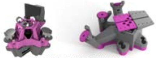
Figure 3: OpenFlexure Microscope and motorized stage [1].
