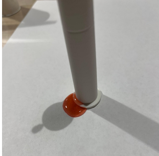
Figure 10. Leakage observed from plunger connection
