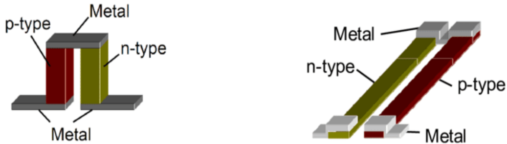
Figure 7. Illustration of a vertical configuration of a thermocouple (left) and of a horizontal configuration of a thermocouple (right) [21].
