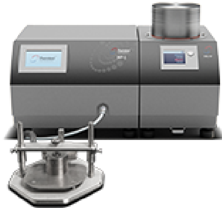
Figure 2: Thermtest MP-1 device for measuring thermodynamic properties of samples [5]
