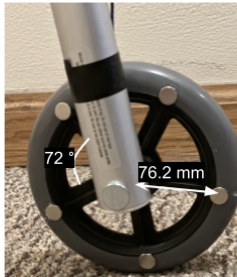
Figure 21: Hall effect sensor & magnet setup
