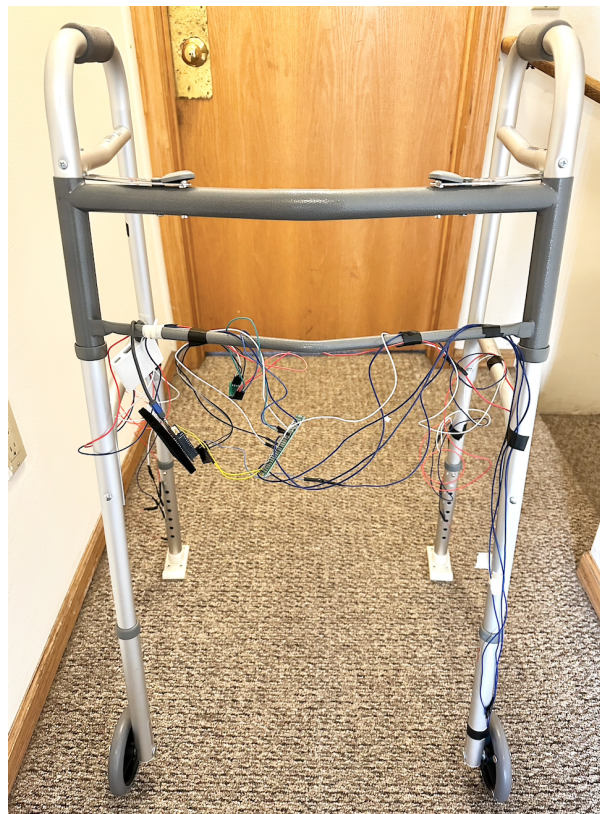
Figure 19: Completed final prototype with sensors, feet, protoboard, and microcontroller
