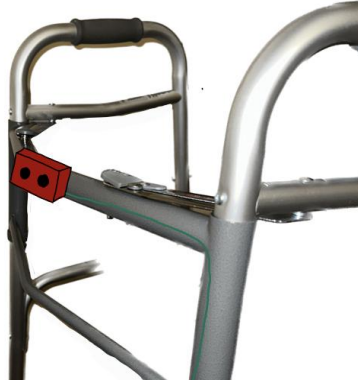
Figure 3: The distance sensor
