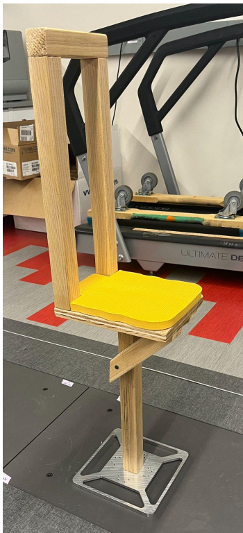
Figure 5. Prototype of the bench with the aluminum base. Dimensions in inches.
