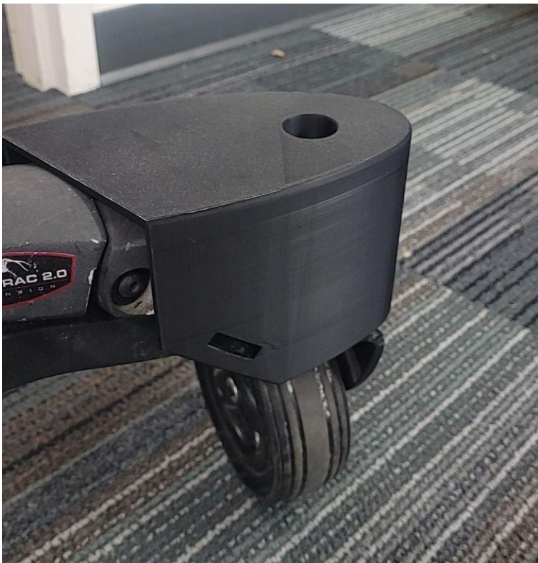
Figure 7: Castor cap inserted into the hole in the castors on the wheelchair
