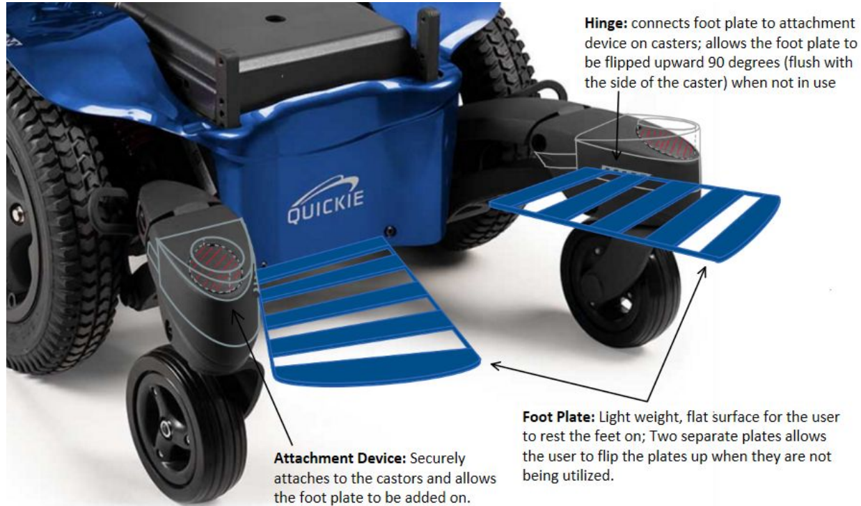
Figure 16: Chosen Preliminary Design- Fold-Up Footrest
