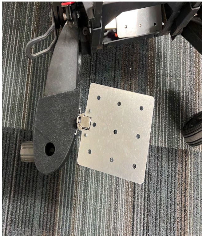
Figure 8 : Final Prototype of castor cap and footplate assembled with a 100-degree hinge from top view.
