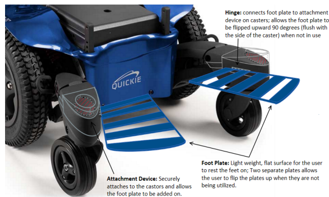
Figure 1: Fold-Up Footrest Design Drawing
