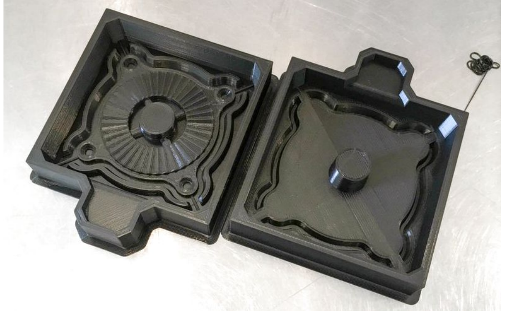
Figure 8: 3D printed molds for resin casting
