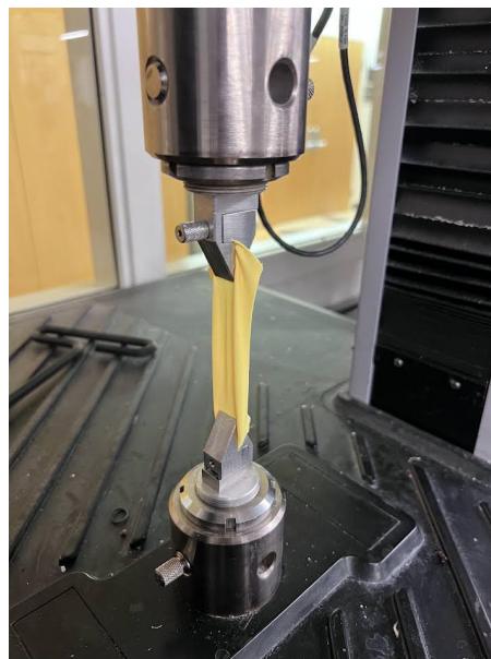
Figure 11: Tendon fabric at the start of tensile test inside of the MTS Machine
