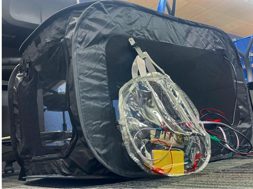
Figure 2: Image of final prototype. For this semester, the electronics were housed within a dog cage that provided an adequate testing environment by having appropriate ventilation and insulation.
