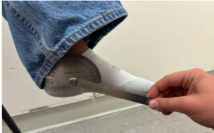
Figure 13: Resting Foot Angle Measurement with Protractor
