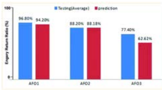
Figure 3. Bar graph comparing the Energy Return Rate (%) results from the bench-top study, in blue, and FEA model, in red, for three different AFOs.
