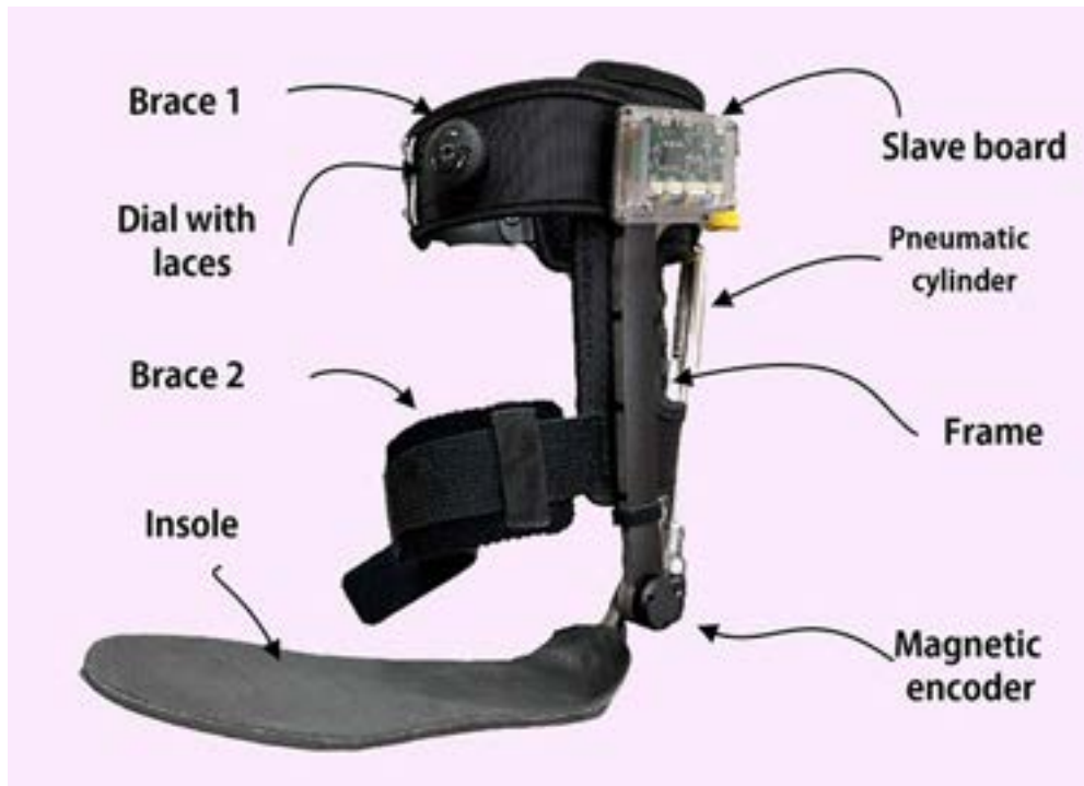
Figure 1: AFO air-compression design [1]
