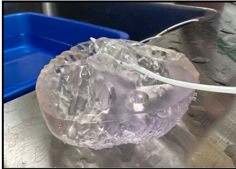
Figure 19: Balloon catheter inflated in pulmonary valve in model
