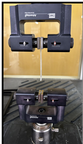
Figure 15: Sample rupture near clamp connection
