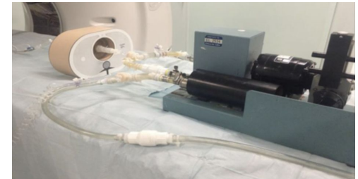
Figure 4: Cardiac perfusion phantom inside the anthropomorphic thorax along with the pulsatile pump [4].
