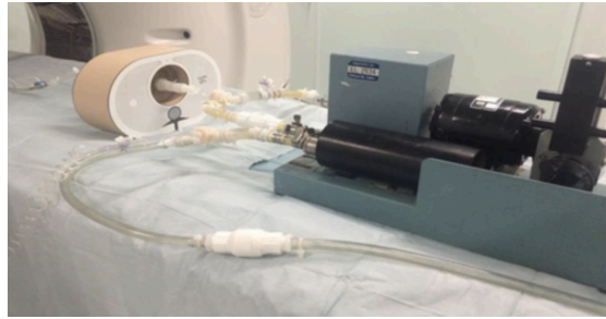
Figure 3: Cardiac perfusion phantom inside the anthropomorphic thorax along with the pulsatile pump [4]
