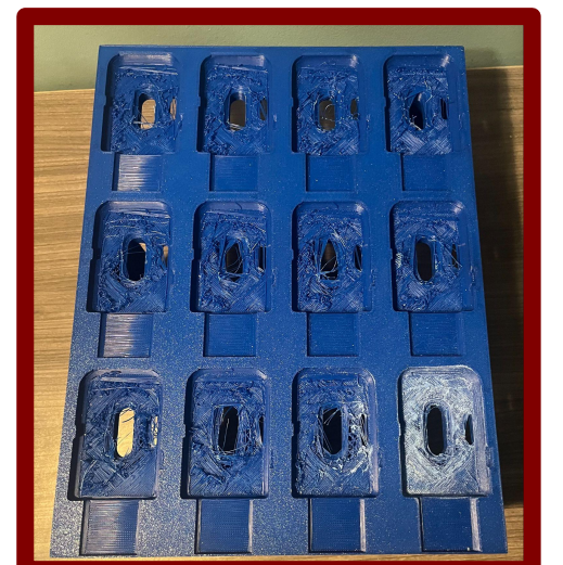
Figure 21: Print Failure of Final Tray Design
