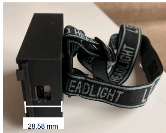
Figure 9: Final light logger design featuring the depth of the box and hole for the microcontroller connection to monitor
