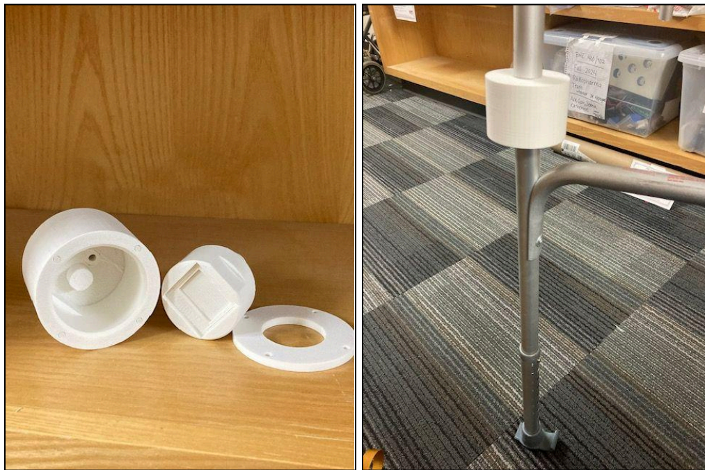
Figures 6 & 7: Image of initial prototype load cell holder (left) and prototype assembled with walker leg (right)
