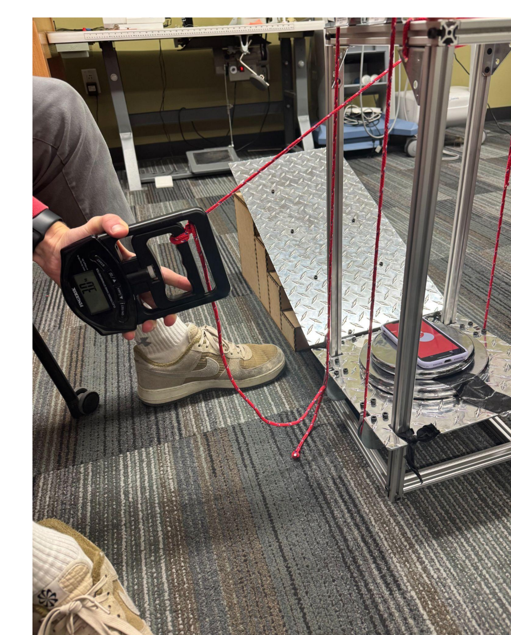
Figure 10: Testing of Required Force and Platform Angle With 7.5 kg Load and Nylon
