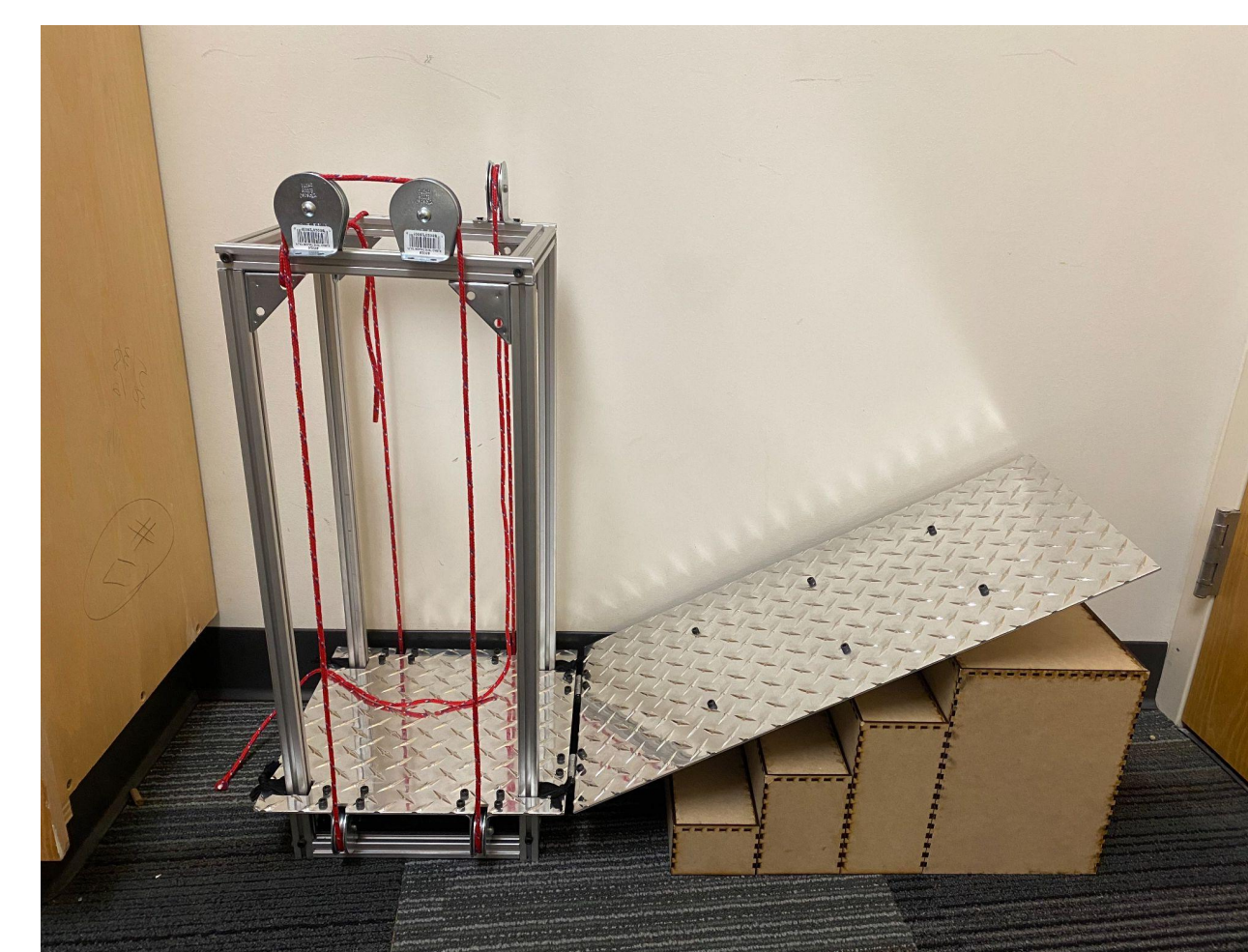
Figure 5: 3:1 Scale Model at Lowered Position
