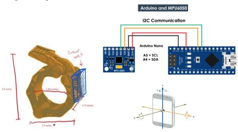
The team will move forward with the 3D printing of a functional weight lifting clip with necessary housing for the following technology. We will utilize an Arduino Nano in each clip, paired with a MPU6050. The arduino nanos will collect data and pair with each other via bluetooth, and the MPU6050 will collect data in terms of angular velocity and acceleration. We will derive this data to displacement, and establish a coordinate system and line of best fit of the barbell path from there.
