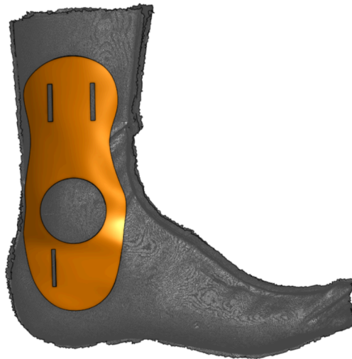
Figure 10: OnShape model of AFO on 3D-printed foot.
