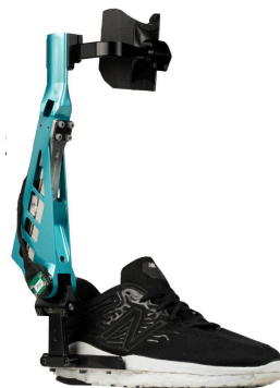
Figure 4: Variable Stiffness AFO (VSO) [4]
