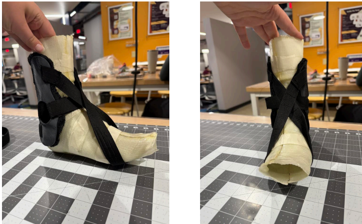
Figure 11 : Finalized prototype to aid in dorsiflexion and prevent ankle eversion and inversion.
