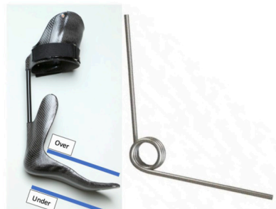
Figure 1: Passive Dynamic AFO (PD-AFO) [1]
