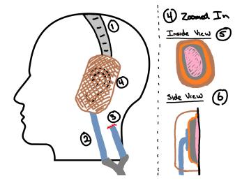
The second concept, the Headphone, focuses on targeted therapy by enclosing only the ear region within a rigid outer shell lined with a soft inner cushion. This over-ear "cup" structure mimics the shape of a headphone, allowing precise control of pressure and easy adjustment of fit through a single head strap. The design offers effective
