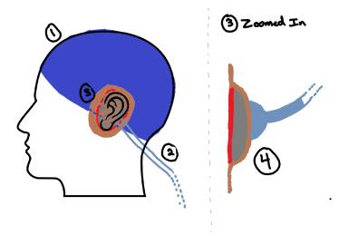
The first design, the Hat, takes the form of a soft, full-coverage cap. Around the ear, a concave surface maintains an airtight seal while conforming to the irregular surface of the reconstructed area. This design ensures a uniform suction environment and stable pressure but may compromise breathability and comfort during long wear due to its full-head coverage.
