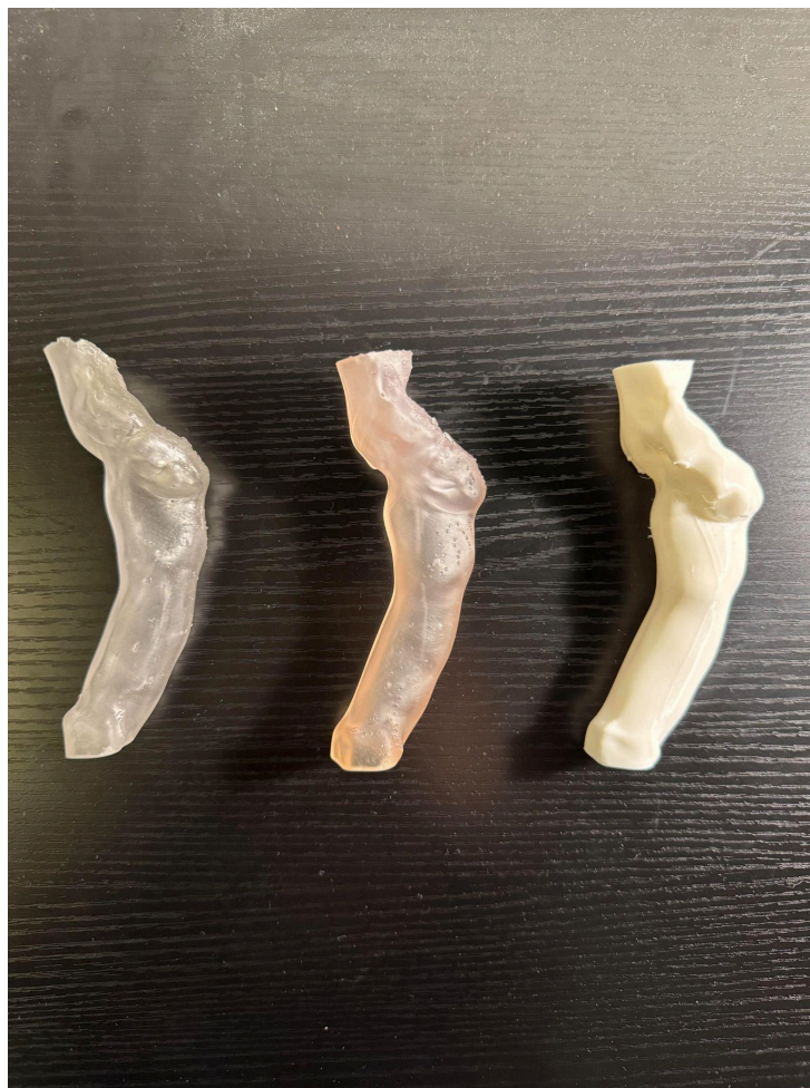
Figure 7: Three Printed Airways, Material from left to right: Elastic Resin, Flexible Resin, TPU
