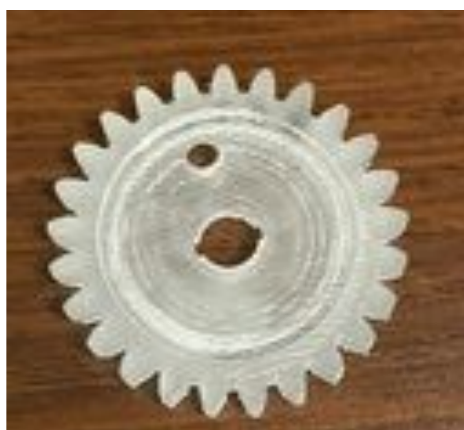
Figure 7: Photo of the integrated rotary element after the durability testing
