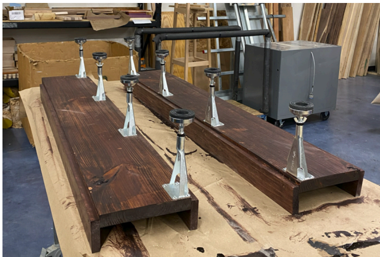
Figure 12: Finished sidetracks with Red Mahogany stain and adjustable legs attached
