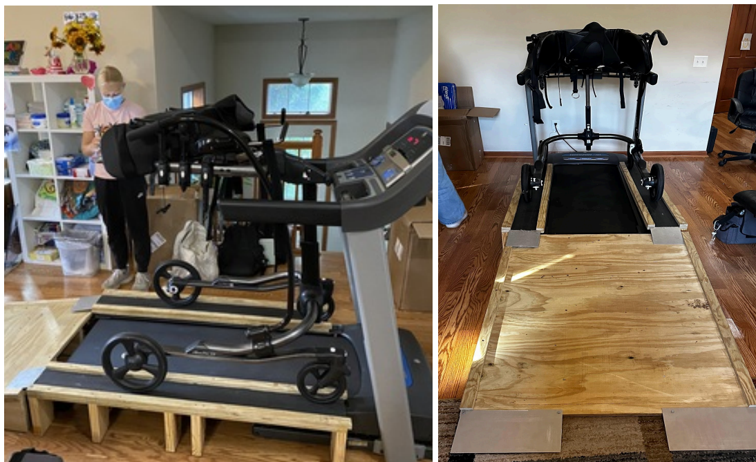
Figure 1. The Fall 2024 fabricated design features wooden side tracks for the gait trainer to rest on top of with a wooden ramp leading up to the treadmill. The images above feature the patient's Rifton Pacer Gait Trainer with the K640 Large Utility Base. The wooden side tracks are built to rest above the side of the treadmill and laterally extend the usable area for the Gait Trainer to rest.
